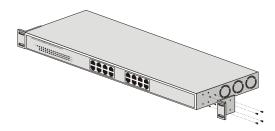
Figure 3-2. Attach mounting brackets with screws
